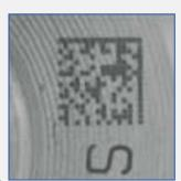
Automotive: mvBlueCOUGAR-X reading Data Matrix codes on plastic components.
