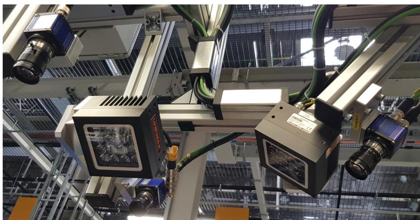
**Figure 1:** The industrial cameras from MATRIX VISION at the plant of the automotive supplier (Station 2). The figure shows several industrial cameras and flat light sources. Because of the long working distances and the light-intensive illuminations required at times, high-performance flat light sources with lens optics were used. (Photos courtesy of MATRIX VISION.)
