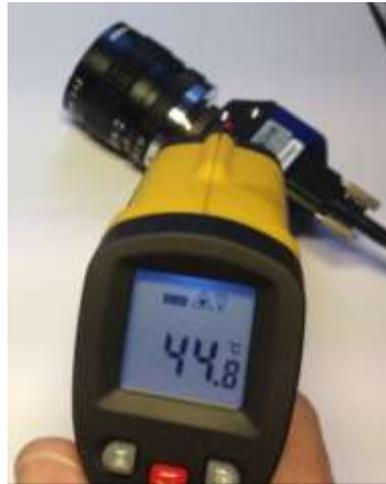
Simply placing the same camera on a heat sink, as shown, can lower the thermal resistance, by conduction and convection, considerably. Here the temperature is measured again at the same spot (used Hold function of unit):
