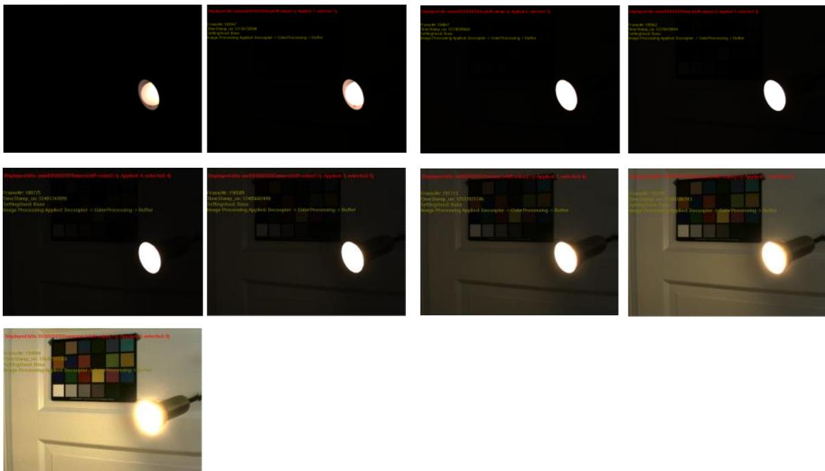
From the left side above to the right side below the image will be shifted downwards by one bit, i.e. the exposure values will be doubled per shift. You are able to see, that the lamp is not overloaded in the higher bits and that you can see the rest of the image in the lower bits.
