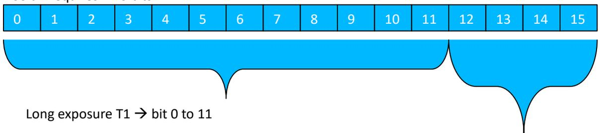
Long exposure  $T_1 \rightarrow$  bit 0 to 11
