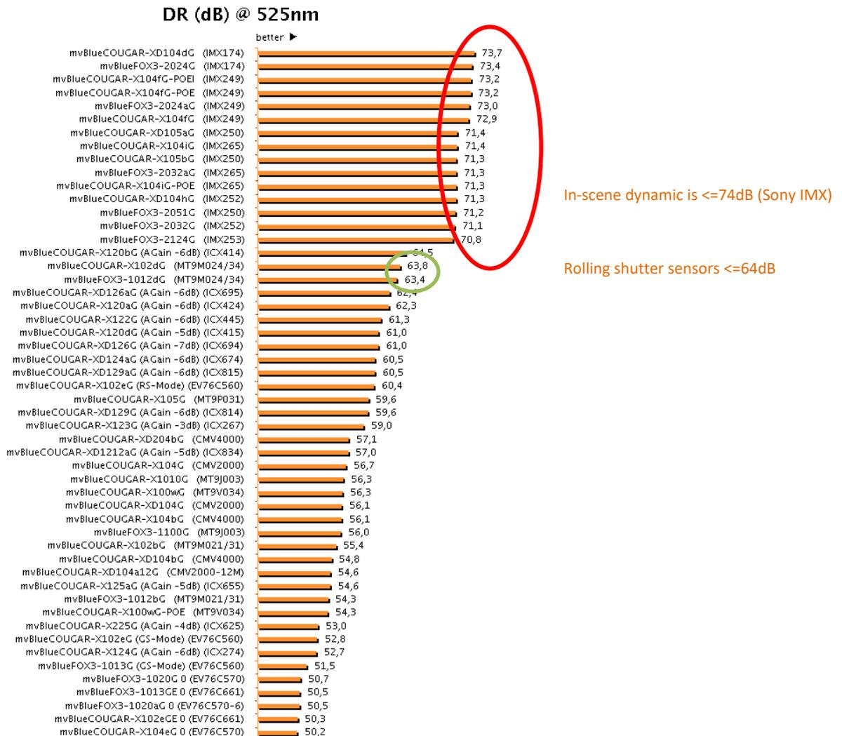
The figure shows that the already legendary Sony IMX sensor of the Pregius series achieves about 70dB, which corresponds to ~12 bit. Furthermore, high-quality CCD sensors from Sony achieve about 60dB (10 bit) and less expensive rolling shutter sensors achieve more than 60dB. At the moment, it is not possible to get more with machine vision cameras.
