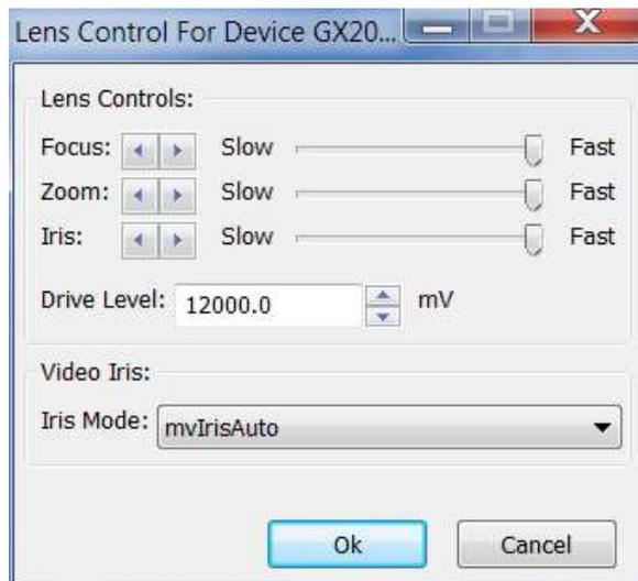
Select the "Drive level" voltage according to the lens type.
