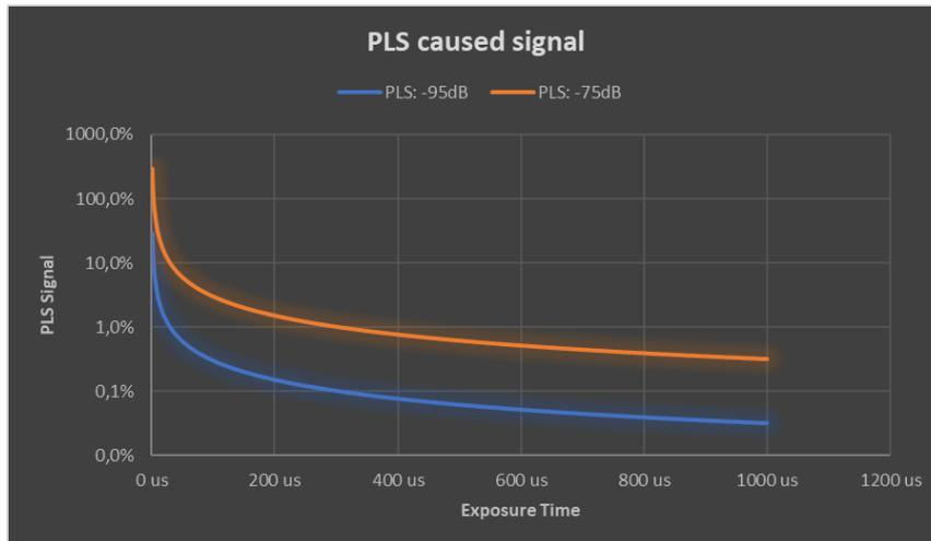
**Figure 2:** PLS caused signal for different PLS values at 60 fps (17 ms) readout speed
