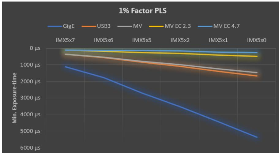
**Figure 3:** Min. exposure time at 1% brightness gradient (Factor PLS) with Sony Gen4 sensor at different hardware interfaces GigE/USB3: max. sensor readout due to the interface limit
