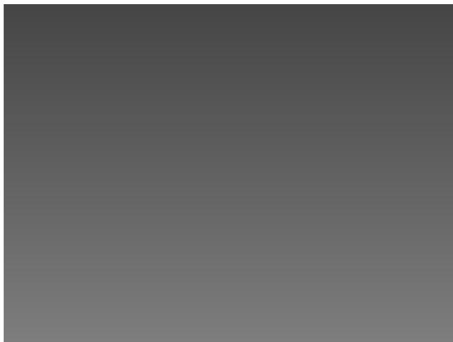
**Figure 1:** PLS caused brightness change in y-direction (in this example 20 % for better visibility)
