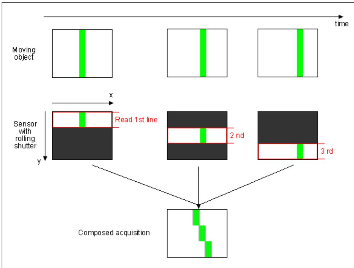
Figure 2: Shifted image during horizontal object movement
