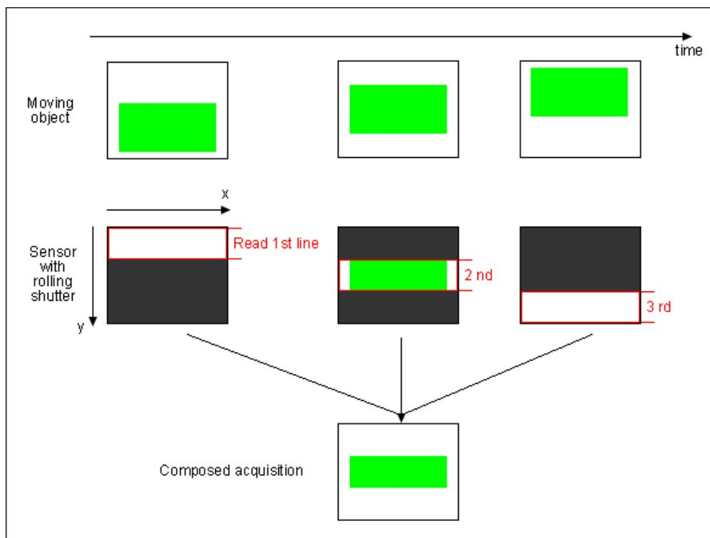
Figure 3: Compression during vertical object movement
