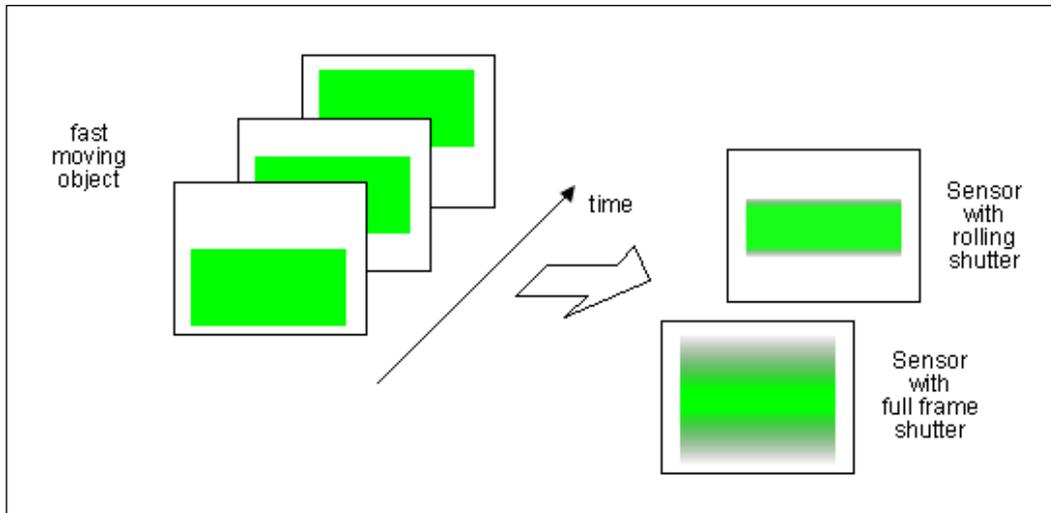
Figure 4: Reduced blur with rolling shutter
