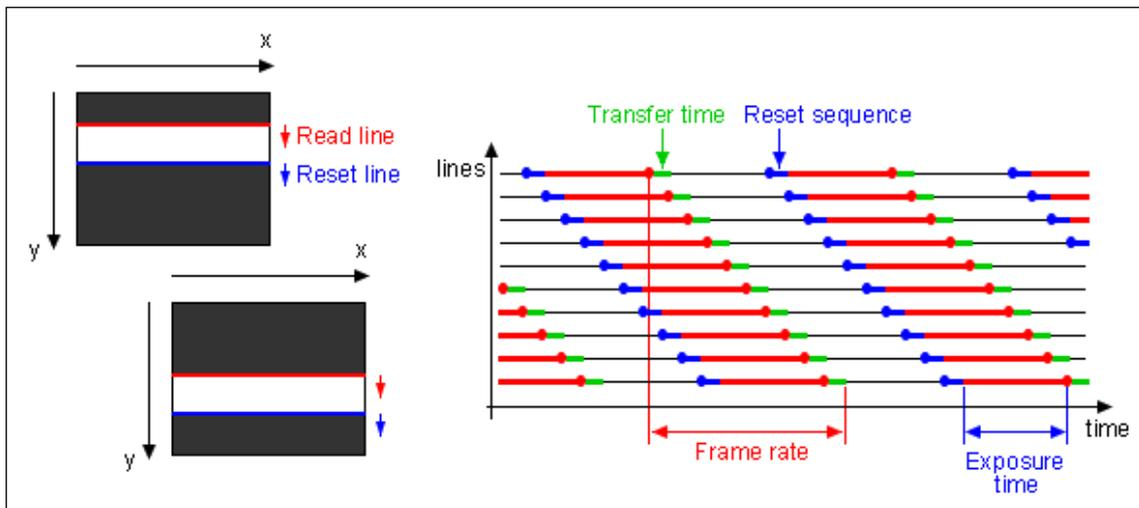
Figure 1: Exposure of every line starts and ends at different times
