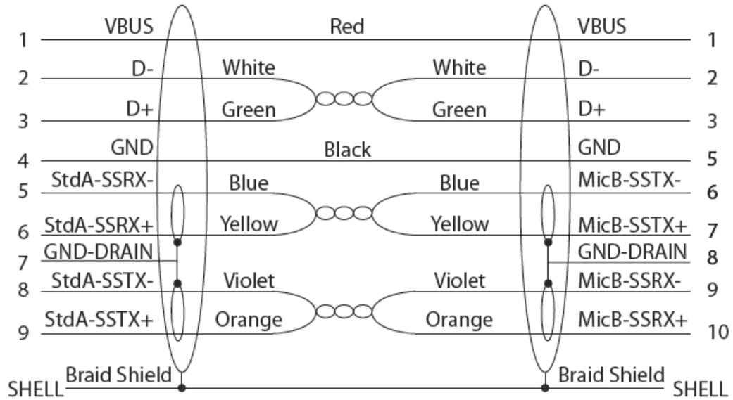
Two wires serve for the VBUS power and its associated GND, one common braid shield is connected to the metal shell and a separate USB 3.0 twisted pair shielding goes to separate pins on the connectors. USB 3.0 signals and grounding in the USB 3.0 camera mvBlueFOX3 series is as follows:
