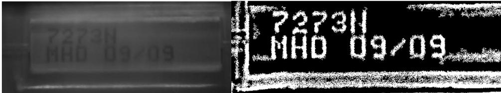
Using a defined area of interest, the camera acquires an image. This image will be binarized and finally an optical character recognition will be performed.
