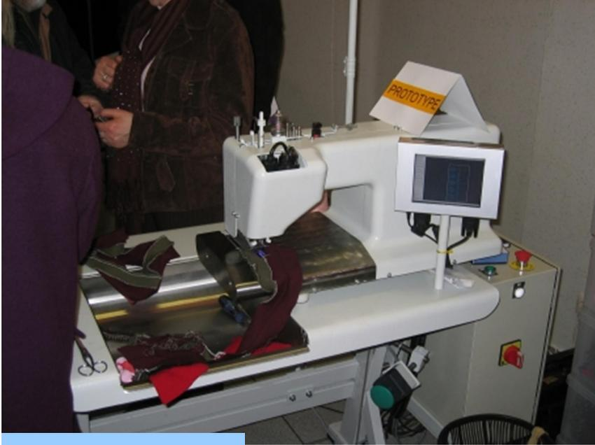
*Figure 1: With the help of industrial image processing a new linking machine replaces 16 standard machines.*
