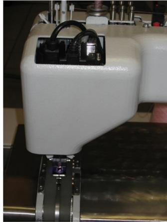
Figure 3: The prototype of the new linking machine works with an integrated mvBlueLYNX camera instead of the eyes of the operator.
