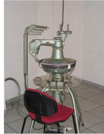
Figure 4: The standard linking machine demands skills and flair by the operator.
