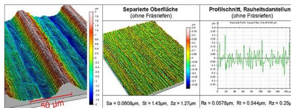
Figure 3: Metal surface with milling grooves (3D-Shape GmbH)
