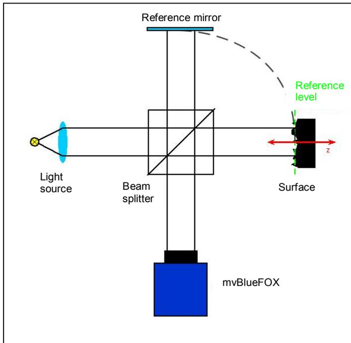
Figure 1: Simplified diagram of the white light interferometer's functional principle.
