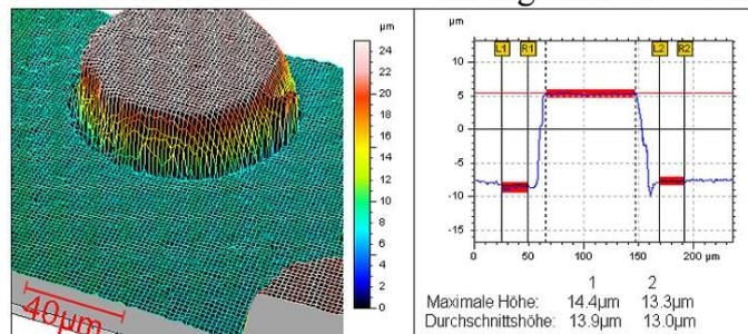
Figure 2: 3D measurement result of an electronic part (3D-Shape GmbH)
