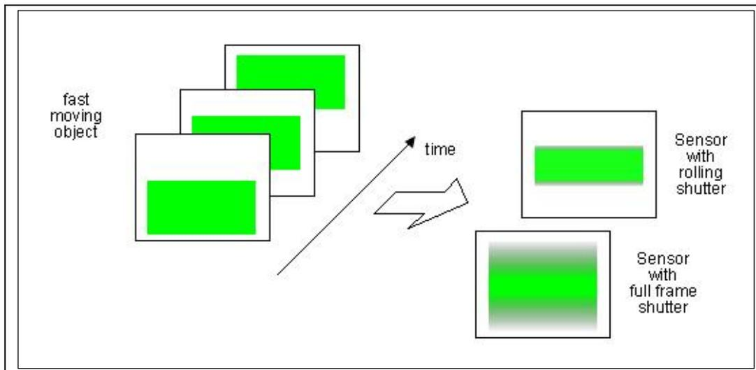
Figure 4 reduced blur with rolling shutter
