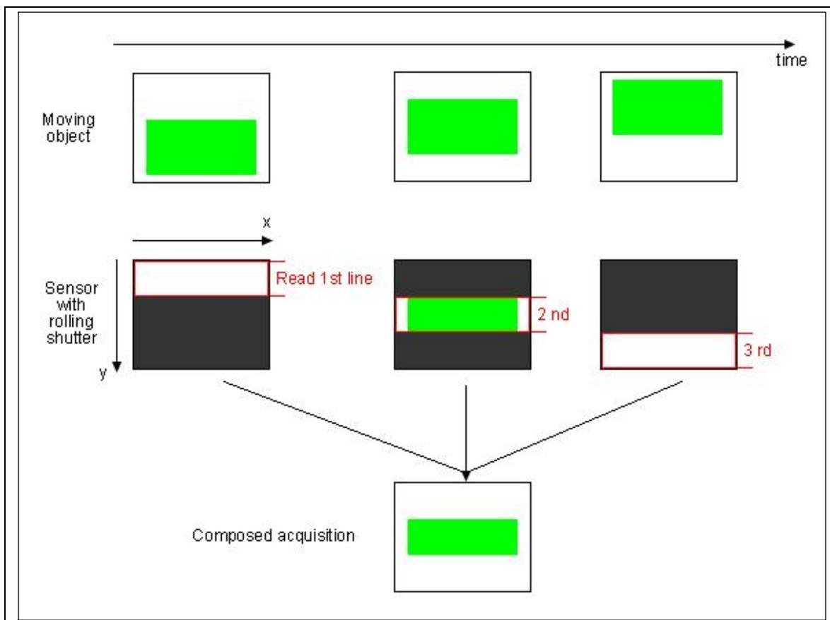
**Figure 3 compression during vertical object movement**
